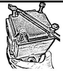
Using a prybar on the bolts, turn the housing making sure **NOT** to lift the housing off shaft end cover.
