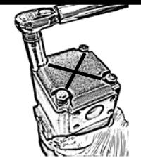
Torque bolts to specifications in a cross pattern.
