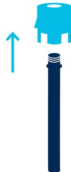
3) Remove the nut at the end of the cable and insert the cable through either the  $\frac{1}{2}$ " or  $\frac{3}{4}$ " antenna mount, based on the size of knockout hole.
