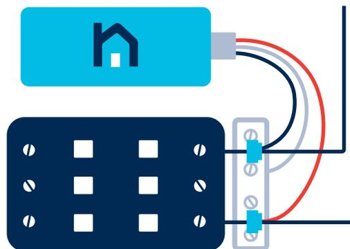
**NOTE:** To find breakers on different phases, you can trace the phase visually. Typically, every other breaker is on a different phase. You can also use a dual pole breaker because they use both phases.
