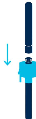
4) Replace the nut on the cable and attach the antenna to the end of the antenna cable.
