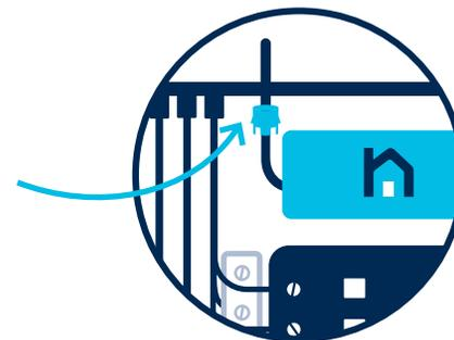
5) With the antenna inserted into the antenna mount, insert the antenna through the open knockout and click the antenna mount in place.
