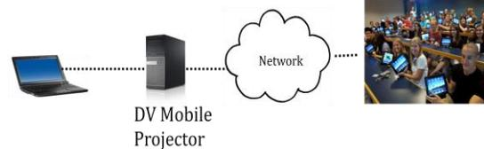
The DVMP takes a "snapshot" of the video input every second and delivers it via an http server to conventional web browsers and the images are automatically updated. To keep wireless bandwidth usage at a minimum, new images are only created when there is a sufficient change in the video source. The delay is approximately 1 to 4 seconds.
